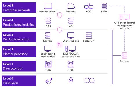
Sensors collect all the data from your OT network and feed it into the management console, alerting you to anomalies and threats. This can also be linked to your SIEM and SOC if required.
